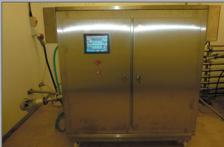
Above: The photo shows the 8 magnetron machine which is designed for small scale production in the region of 100-300 L per hour. The flexible system has many potential applications and so far has been adopted for the pasteurisation of juices and the production of sauces.
