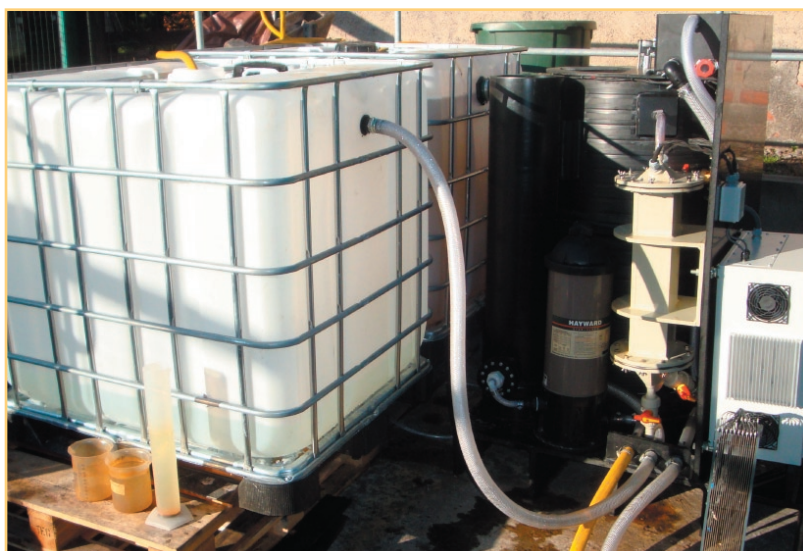
Above: Test rig for removing copper from waste water.
