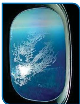
**The Build of Ice Crystals and Supercooled water at altitude can be extremely hazardous to the operations of aircraft. NRC sensor technology, enabling better detection of ice crystals on board aircraft, will be tested by the HAIC programme.**
