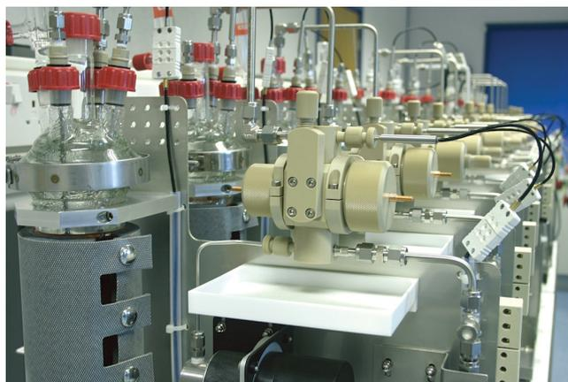
*“Routine corrosion testing to evaluate a matrix of parameters is extremely time consuming. The ACT multi-cell approach provides the potential for significant benefits and savings by enabling true parallel testing to be carried out in highly controlled environments”.*
