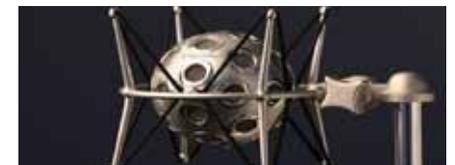
**An Eigen Mic, a spherical microphone that can be used for recording spatial audio signal.**
